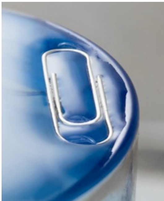
Figure 1(at right): The surface tension of water carries the weight of a paper clip (source: Wikimedia Commons)
